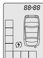
*As soon as the Power Save mode is activated the respective icon will appear on the LCD panel meanwhile all the remaining symbols will disappear.*
