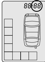
Once the Hours have been confirmed by pressing button 3, the minute's digits will start to flash. Use the same buttons to change the minute's digits and when the minute's digits are confirmed, then the time will be set and the display will return to a standard display format and the transceiver will emit a clock set melody.
