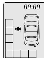
The LCD Display includes a transceiver battery discharge indication. When the transceiver battery voltage becomes less than 1,3V the exclamation sign will be flashing on the LCD panel. When the battery voltage is less than 1,2V audible confirmation on pressing the button and all audible/vibration indication will be turned off. The LCD indication will continue to operate as normal. As soon as possible replace the battery to reinstate the alarm system protective abilities in full.
