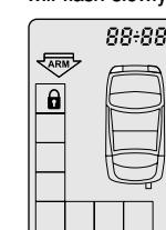
*The LCD Transceiver will confirm the alarm system is armed with a beep, and the LCD screen will display an armed state.*
