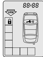
The Shock Sensor Icon on the LCD screen will be solid on during entire period of the Sensor Override Mode.
