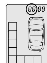
The Hour's digits will start to flash. Press Button 1 to increase the hours by 1 hour per press and Button 2 to decrease the hour by one hour per press. Press button 3 to confirm that the hour's digits are correct.
