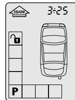
The LCD Transceiver will confirm the alarm system is disarmed with two beeps, and the LCD indication will change to disarmed state indication.
